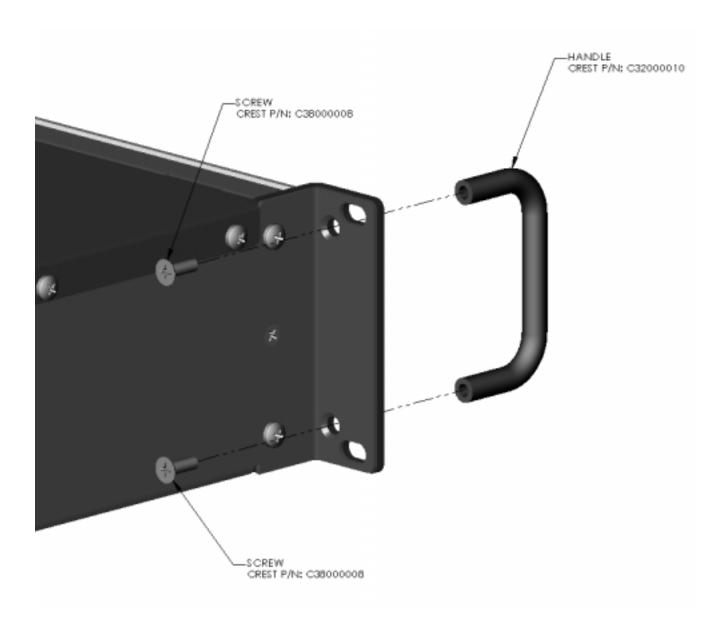
The CD amplifiers can be outfitted with optional handles. This option requires (2) CD series handles (P/N C32000010) and (4) #8-32 1/2" undercut flat head screws (P/N C38000008). You may order these from your dealer or directly from Crest Audio.
